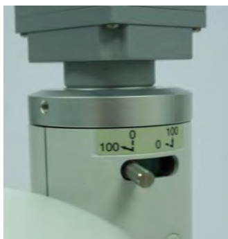
Optical path switching lever position for microscope viewing
