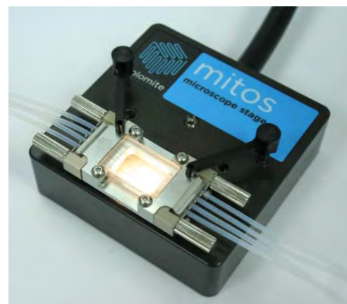
Chip placed on microscope stage
