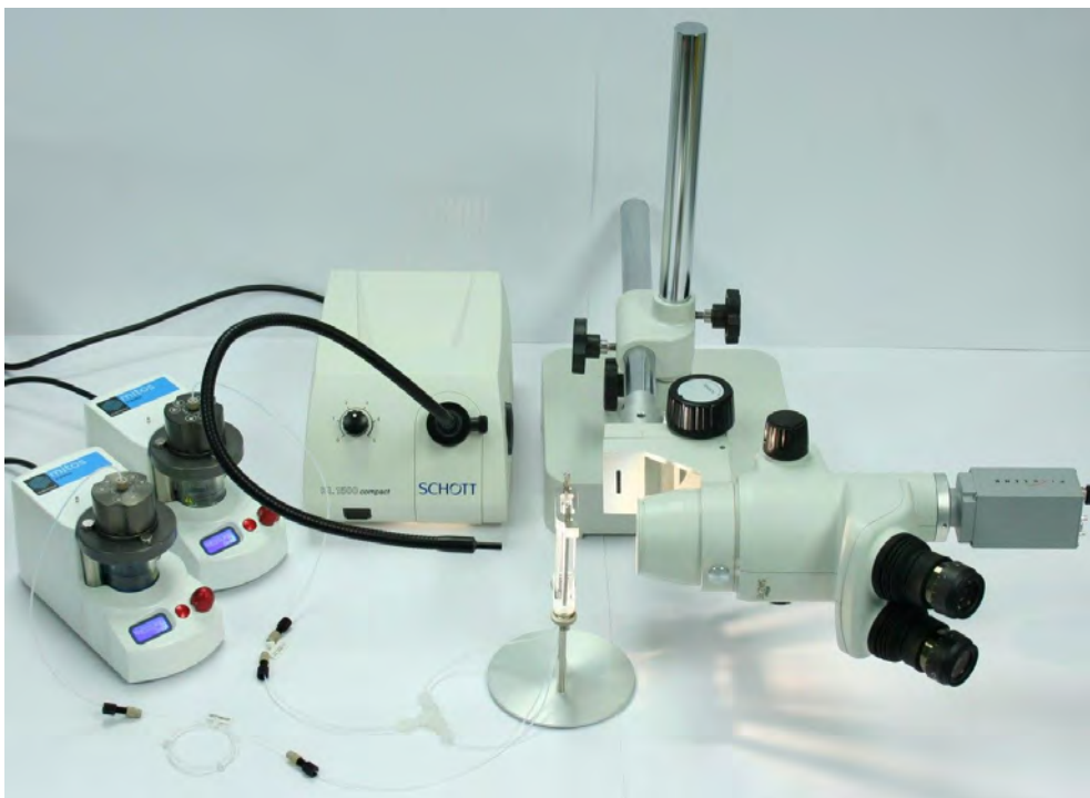
High Speed Camera and Microscope System in use with the Droplet Emulsion System
