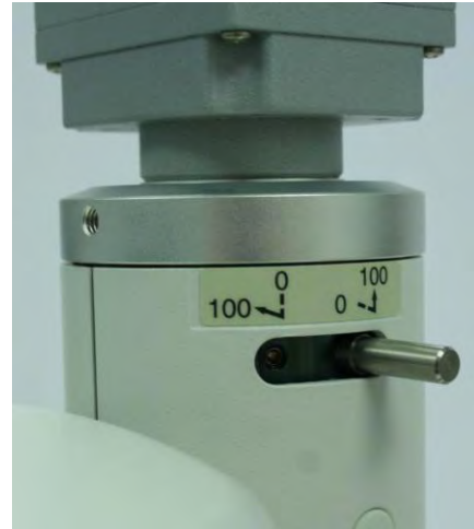
Optical path switching lever position for camera use
